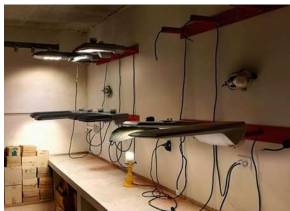
Fig. 5. Aspects of 6,000 h operation test (photo from author)
